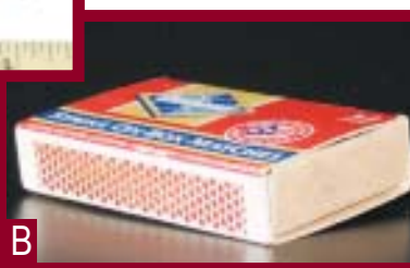
Figure 1: Red phosphorus is easily recognizable as a dark red to purple solid powder [A]. It can be obtained from scrapings off match box strike plates [B] and other incendiary products or from commercial chemical supply companies [C]. Photos Courtesy of CA Department of Justice. Photographer, Charles Salocks.
