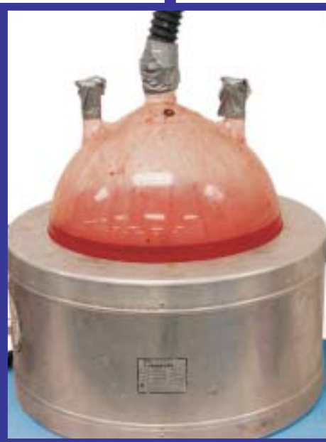
Figure 1: Photo of a heat-resistant vessel containing a hydriodic acid / red phosphorus methamphetamine synthesis reaction mixture. Phosphine gas is an unwanted potentially lethal by-product generated during the synthesis. Phosphine may be present in the air space above the liquid reaction mixture. Photo Courtesy of CA Department of Justice.
