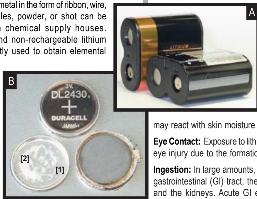
Figure 1: Lithium is a light-weight silvery colored metal used to synthesize methamphetamine. It is collected from camera batteries [A] and other small button type batteries [B]. Once these batteries are broken open, the lithium [B.1.] immediately begins to react with air [B.2.]. Photographers, Charles Salocks and Caron Poole.
