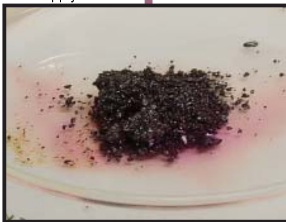
Figure 1: Pure iodine crystals, heated slightly, showing some solid iodine escaping directly to the air as obvious violet-colored vapors. Because of this "sublimation" property, exposures include dermal contact with solid crystals and inhalation of vapors which may not be quite as visible as this at room temperature. Photographer, Charles Salocks.
