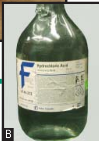
Figure 1: Anhydrous hydrogen chloride gas is stored as a liquid in pressurized containers [A]. Aqueous solutions of hydrogen chloride are called hydrochloric acid or muriatic acid [B] and are found in commercial chemical or swimming pool supply houses. Photos: Courtesy of CA Department of Justice.
