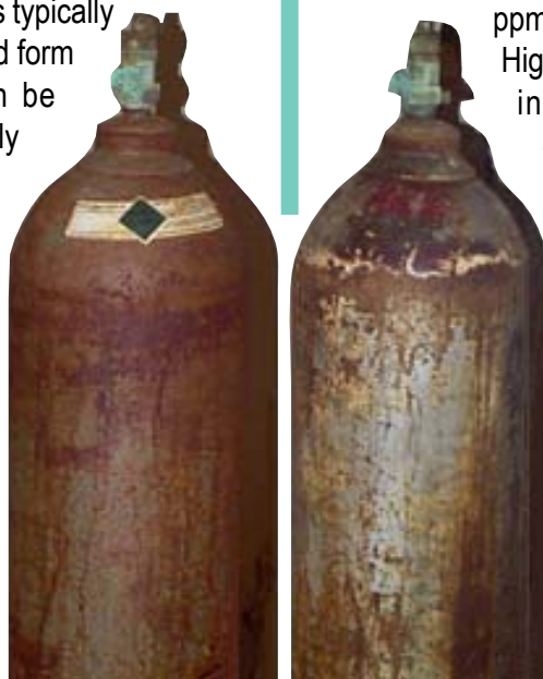
Figure 1: Anhydrous ammonia gas is stored and transported as a liquid in pressurized gas containers. Note greenish-blue corrosion on valves and fittings. "Secondary" containers such as these were not designed to hold ammonia and may fail at any time. Photo Courtesy of CA Department of Justice.
